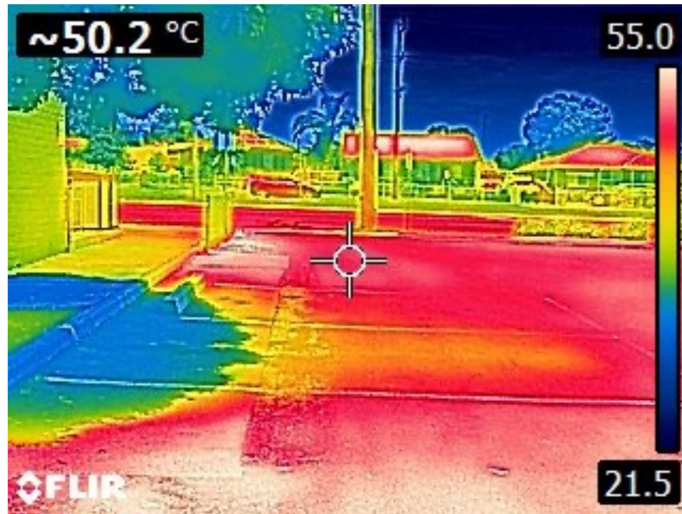
Image 8: Thermal image of Seymour's IGA Supermarket carpark showing the temperature difference between exposed concrete and tree shaded concrete
